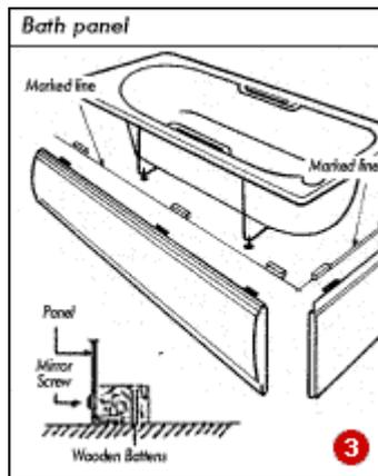
Fit the bath panels according to the manufacturer's instructions (3). Use a fine-toothed saw to shape the panels around pipes or to fit the skirting.
