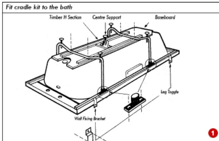
Attach the wall-fixing brackets to the underside of the rim-support frame. Fit hand grip(s) to the rim if supplied.
