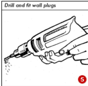
Drill and fit wall plugs on the marks (5). Just drill pilot holes for the screws when fixing to a wooden floor.
