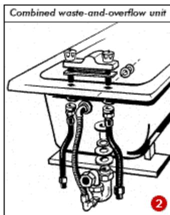
Fit the overflow outlet and waste outlet into the bath. Connect them with a combined waste-and-overflow unit that incorporates a deep-seal trap (2).
