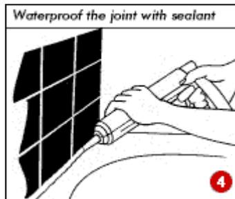
Once the walls have been tiled (4), waterproof the joint around the rim of the bath with silicone sealant.
