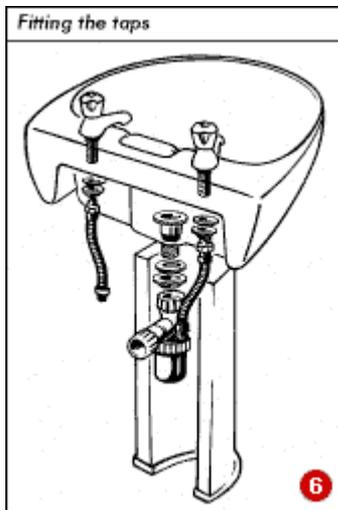
Place the basin on its pedestal and fix it in place with brass screws. Connect the trap to the existing 32mm (1.25in) wastepipe. If a new waste pipe is required in a different position, drill a clearance hole through the wall with a masonry core drill, and install a new pipe run (see next section).
